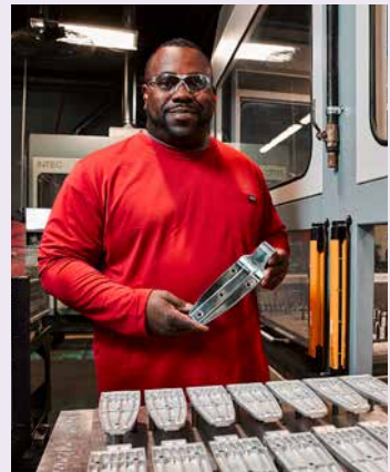
A Kason 1248 Hinge just after robotic polishing.
