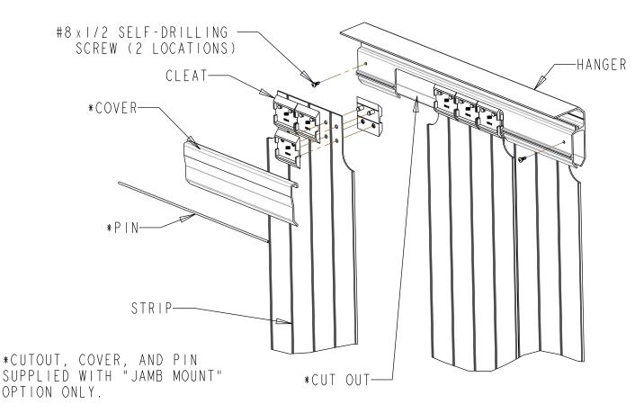
The Maximount hanger can be mounted against the wall or within the opening.
