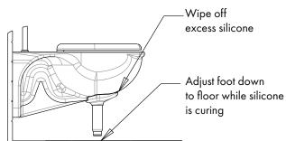
Adjust foot up after it is fully cured
