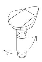
69000TJ3000 leg pivots, loosen and tighten with allen wrench
