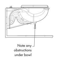
Remove insert when installing on bowl with obstruction
