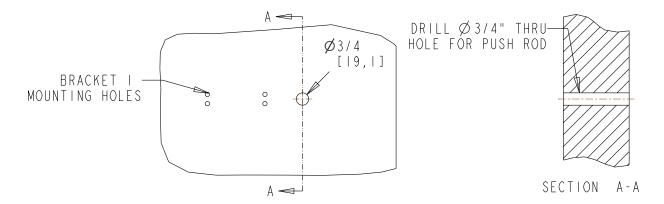
5. Install bracket 1 and 2 with 1/4-20 structural hardware (not included).
