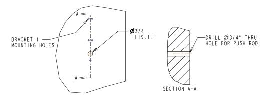
5. Install bracket 1 and 2 with 1/4-20 structural hardware (not included).
