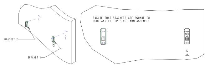
6. Install pivot arm assembly and push rod on brackets 1 and 2.
