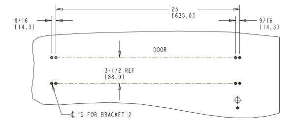
3. Place bracket 2 on door, align mounting holes with drawn centerline, square with edge of door at distance shown, mark centers of slots and center punch (4) holes.
