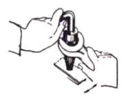
Remove tool from Rivnut by revolving entire tool in counter clockwise direction
