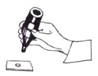
Turn nut the required number of turns or until firm resistance indicates complete upset of the Rivnut (Note: A box end rachet wrench will speed up this operation)
