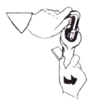
4. Break nut loose with clockwise movement. Remove both wrenches from the tool
