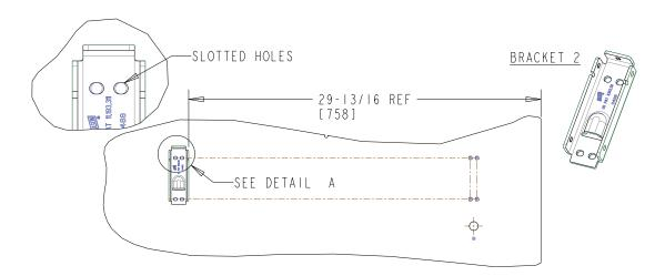
4. Drill a 3/4" diameter (19.1 mm) hole through door. Hole must be square to door surface for proper alignment and operation. At this time, drill holes size appropriate for self-threading structural 1/4-20 screws or 1/4-20 type bolts.
