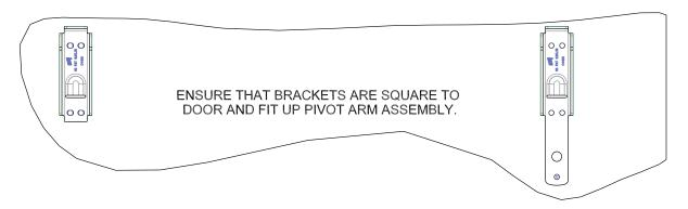
6. Install pivot arm assembly and push rod on Brackets 1 and 2.
