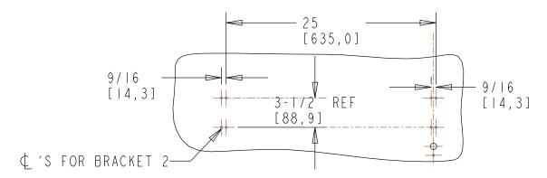
3. Place Bracket 2 on door, align mounting holes with drawn centerline, square with edge of door at distance shown, mark centers of slots and center punch (4) holes.
