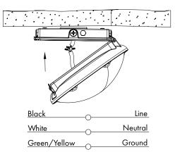
5. Arrange the internal wiring, close the lamp body along the rotating axis, and fasten the side buckles.
