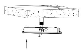
Connet the lamp body back to bottom cover through shaft; Connect the junction box ground to the ground terminal.
