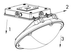
2. Pull the supply wires through the center hole of the bottom cover. Attach securely.
