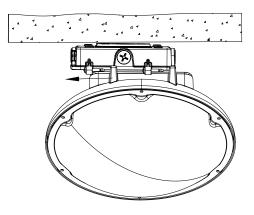
Connect the mains input wire to the power input wire of the lamp accordingly: White for N; Black for L; Green/Yellow for ground wire (GND).
