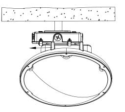
Connect the mains input wire to the power input wire of the lamp accordingly: White for N; Black for L; Green/yellow for ground wire (GND).
