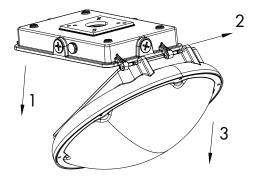
2. Pull the supply wires through the center hole of the bottom cover. Attach securely.
