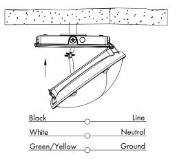
5. Arrange the internal wiring, close the lamp body along the rotating axis, and fasten the side buckles.
