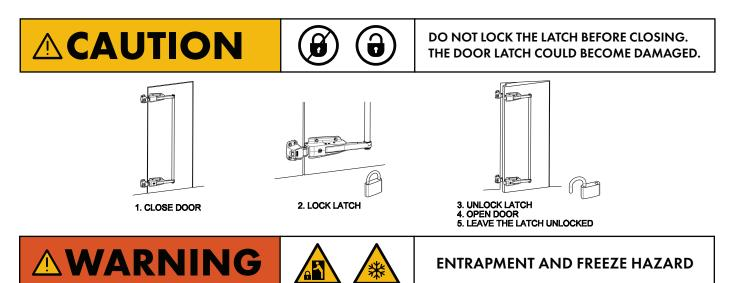
Failure to follow the installation and testing procedures may result in personnel being entrapped and subject to extreme cold, freezing temperatures, and possibly death.
